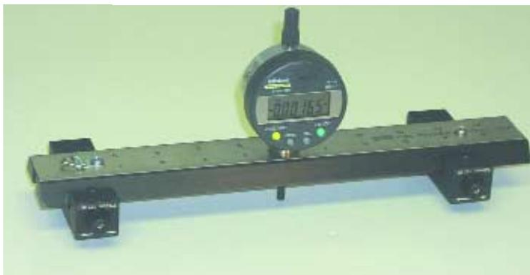
Figure 5. Three-point roll wave gauge with digital readout
